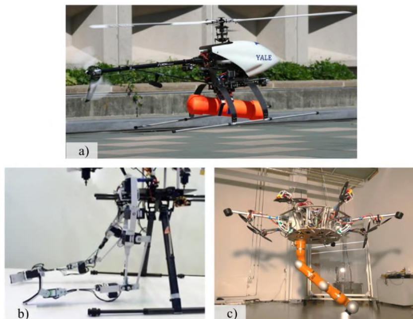
Fig. 48. Types of aerial manipulators: (a) 1-DoF gripper, (b) two multi-DoF robotic arms, (c) cable-suspended manipulator
