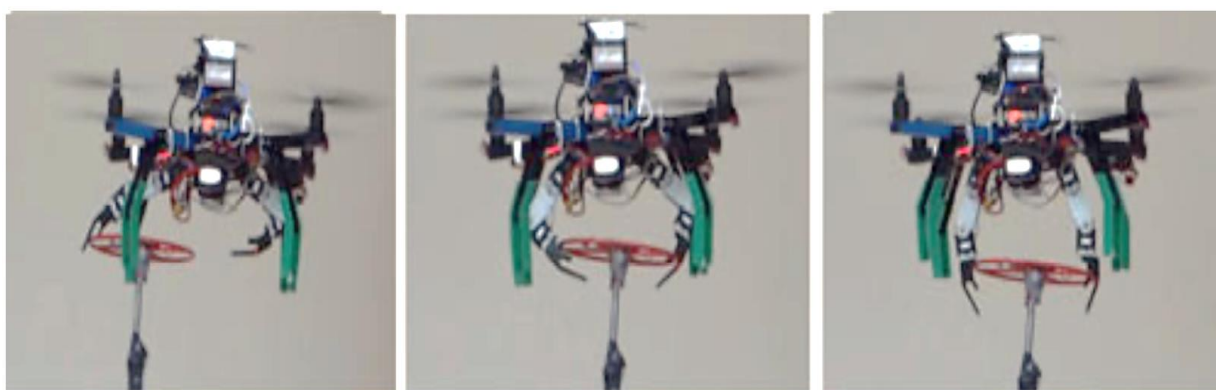
Fig. 39. Quadrotor UAV Autonomous Valve Interfacing Task [5]
