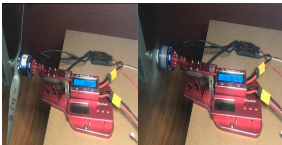
Fig. 19. Experimental device for reverse thrust test of pro thrust test of propeller motor
