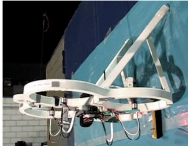
Fig. 15. An unmanned aerial vehicle with a fixed brush tool on the side deployed for window cleaning
