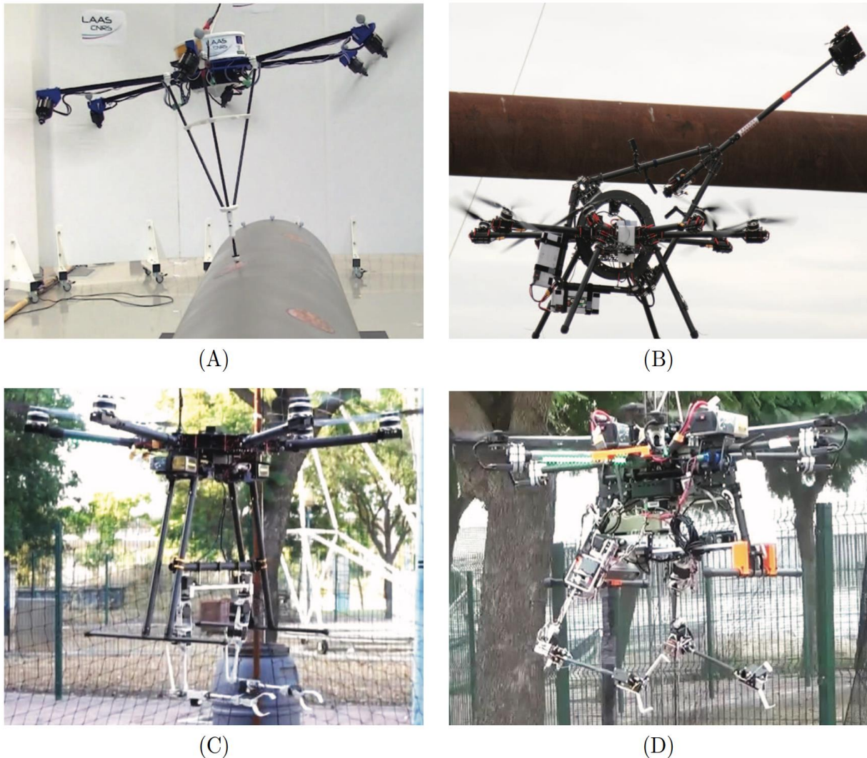
Fig. 40. Four AEROARMS platforms: (A) multidirectional-thrust hexarotor with a rigidly attached end effector, (B) multidirectional-thrust octorotor with inspection arm, (C) aerial dual-arm manipulator with stiff joints, and (D) aerial dual-arm manipulator with compliant joints [6]
