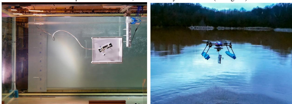
Fig. 22. (Left) The robot is remotely manoeuvred into a confined space with a side opening of 30 cm (Right) The flying dual-robot platform shown during a take-off
