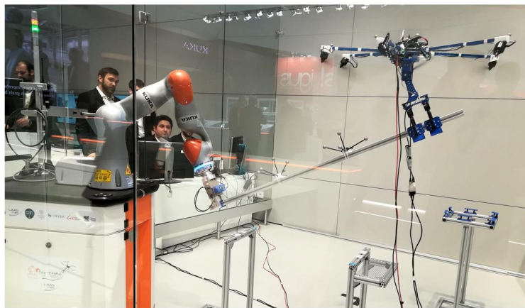
Fig. 40. A snapshot of the cooperative manipulation state of Tele-MAGMaS using bilateral tele-operation approach performed during the KUKA 2017 Innovation Award at the Hanover Fair
