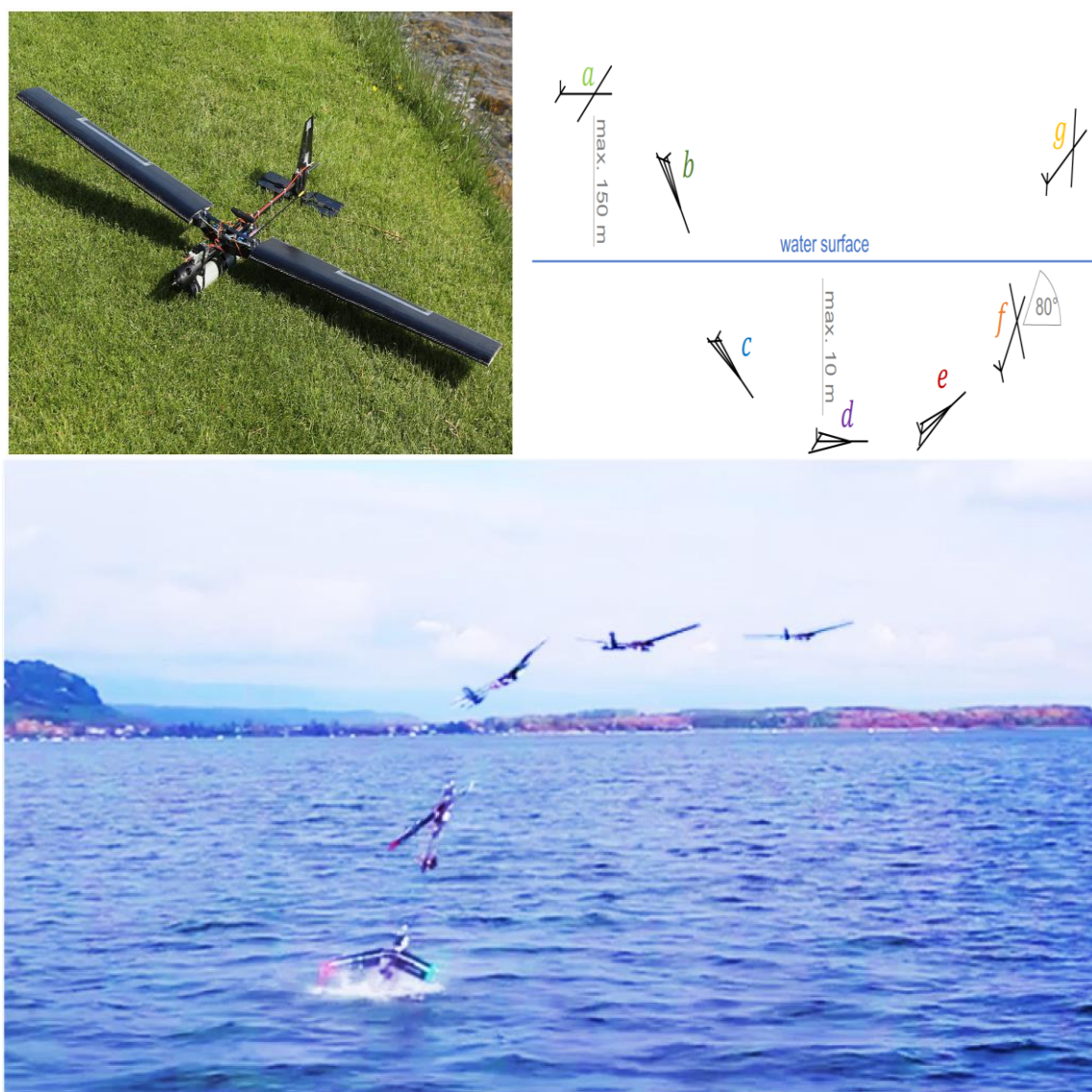
Fig. 11. (left up) Prototype in flight configuration; (right up) Full cycle of flight (a), dive (b; c), swim (d; e) and emersion (f; g); (down) Emersion phase (f; g) followed by flight (a)
