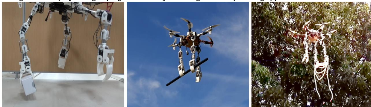
Fig. 49. Grasping objects using the manipulator's gripper. (From left to right) Grasping a small cuboid object using single gripper, a long pipe using two grippers and a bundle of rope being carried between two grippers
