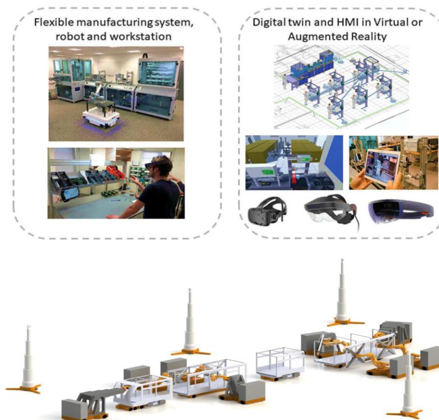
Fig. 1. Flexible manufacturing system and its digital twin [2,3]
