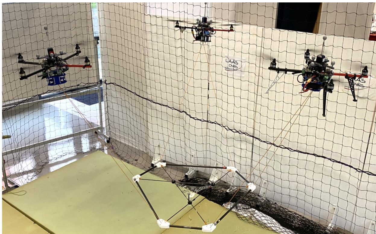
Fig. 35. Experimental screenshot of the Fly-Crane flying while controlling the platform in full pose (position and orientation)
