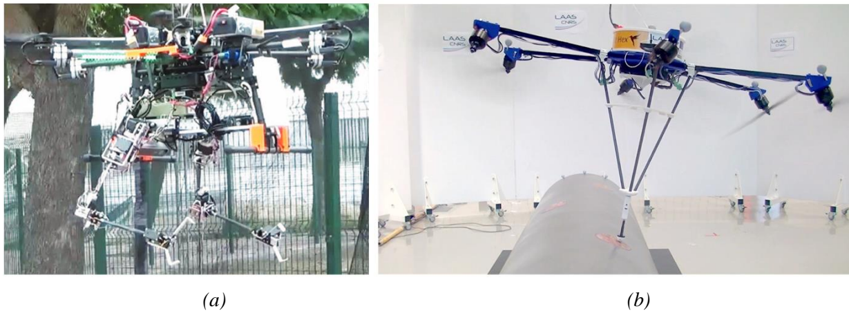
Fig. 31. Second generation of aerial manipulators: (a) An aerial dual-arm manipulator with compliant joints; (b) A fully actuated platform interacting with the environment
